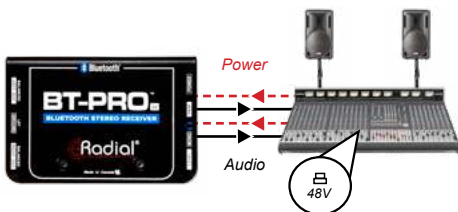
Powering the BT-Pro using 48V phantom power
