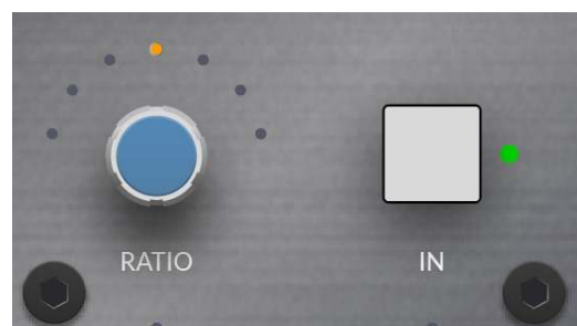
Bus Compressor IN controls plug-in Bypass
