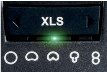
Figure 1: Polar pattern selector
