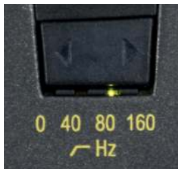
Figure 3: Bass Cut Filter
